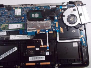
• Next, carefully remove the sliding connector that connect the CPU Fan and the laptop together using the <u>tweezers</u>.
