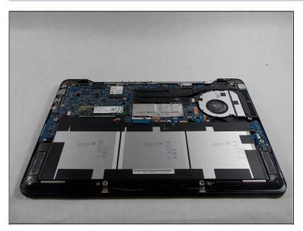
• Locate the battery near the bottom.
