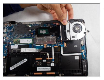
Remove the CPU Fan and Heatsink by simply lifting upwards.
