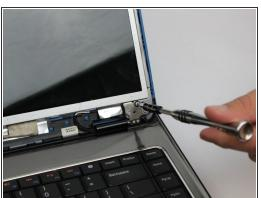
• Using the #0 Philips head, unscrew the screen bracket from the base of the laptop.
