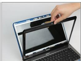
Use a plastic opening tool to remove the screen bezel.
