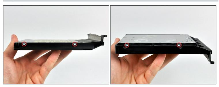
Remove the two 6.5 mm T10 Torx screws from both sides of the optical drive (four screws total).
