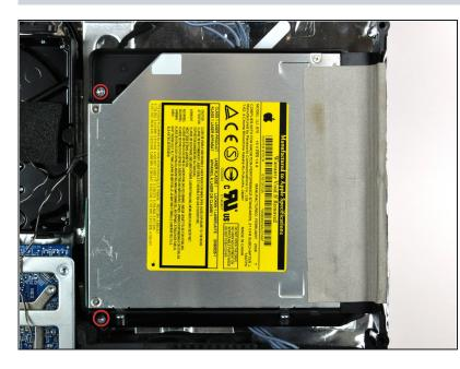
Remove the two fine-thread 7 mm T10 Torx screws securing the optical drive to the rear case.
