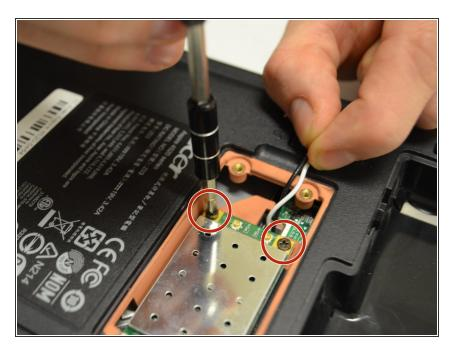
Remove the two 0.5mm Phillips #1 black screws located on the WiFi card.
