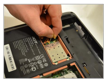
Remove both the black and white wires by pinching the brass connectors and pulling up.
