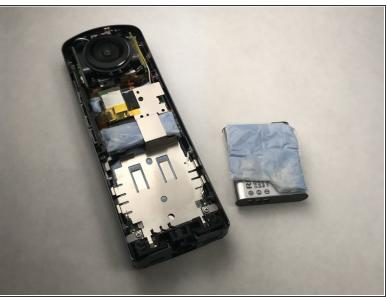
Lift the battery out of the device, beginning with the end closest to the camera.
