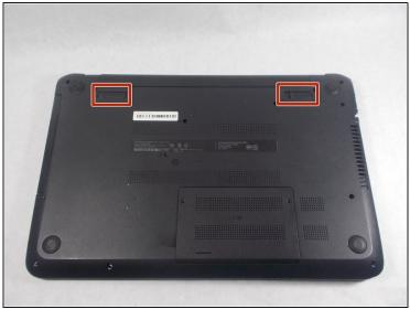
Locate the battery and the two switches that release the battery when they are unlocked.
