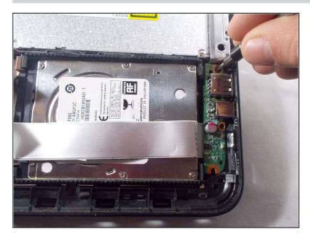
Remove metal bar on top of the CD drive. Do this by removing 3 mm PH1 Phillips head screw that is just below the bottom right corner of CD drive.
