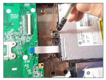
Remove the 3 mm PH1 Phillips head screw that is just to the left of the CD drive.
