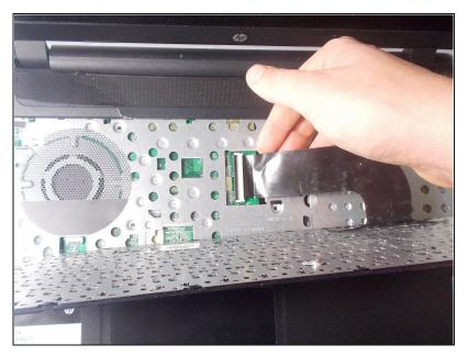
Remove the keyboard connection from the laptop by flipping up the black tab on the ZIF connector.
