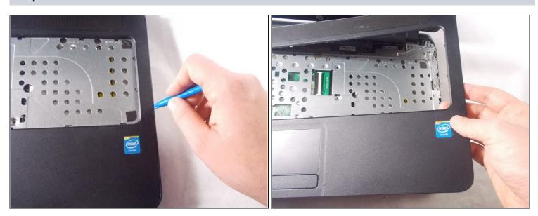
Remove the palm rest using the blue spudger tool.
