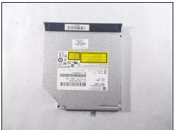
Carefully push the CD drive from its left side out of the laptop.
