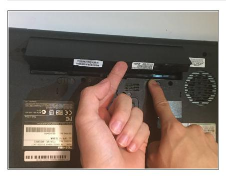
Carefully remove the battery from the laptop.
