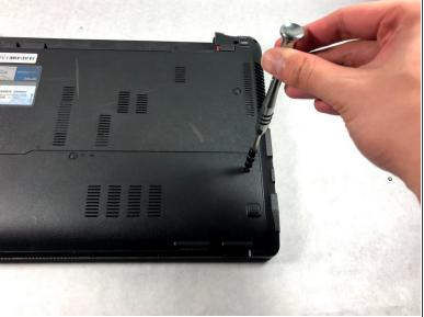
• Use a Phillips #000 screwdriver to remove the two 9mm screws from the HDD/RAM cover panel.
