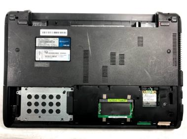
Slide the back panel off by placing a hand on each corner and pulling the panel towards you.
