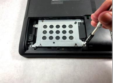
Remove the four 9mm screws holding the hard drive in place.
