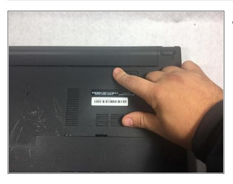
Slide the battery latch all the way to the left until you hear the click and see the battery prop up.
