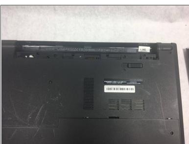
Rotate the battery up and remove it.
