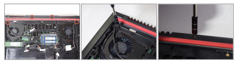
Using the Philips #1 screwdriver, unscrew the 4 x 2mm x 5mm screws, located on the top of the laptop.
