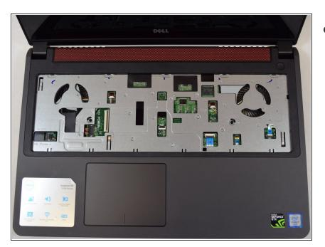
Now that the keyboard has been fully disconnected from the laptop, lift it off of the device.
