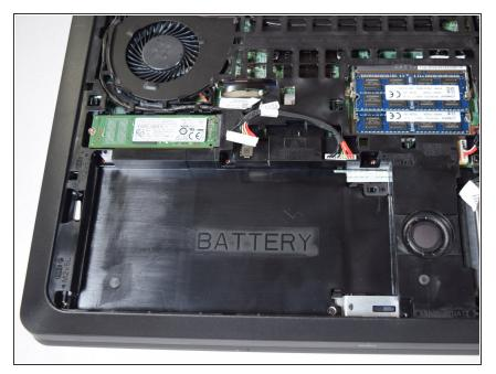
• Now lift the battery from the device to remove it.
