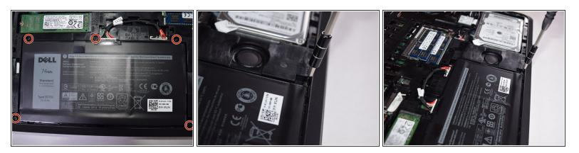
Unscrew the 5 x 2mm x 5mm screws, using the T8 Torx screwdriver.
