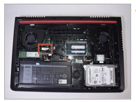
• Locate the LCD cable, near the center of the laptop.
