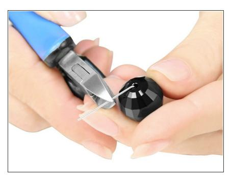
Use side cutters to cut the wire, leaving a tail that's about one third of an inch long.
