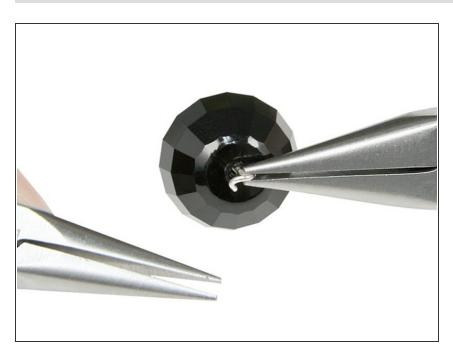
To open and close the loop, you can use chain nose pliers and gently twist it open from side to side.
