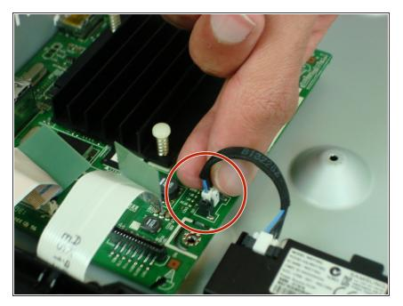
Disconnect the WiFi board cable connector from the main logic board
