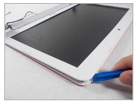
• Pry off the face panel on the screen using the blue prying tool.
