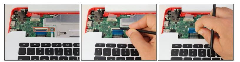
Disconnect the two ZIF connectors by prying up the locking bar with a spudger and removing the ribbon cable.
