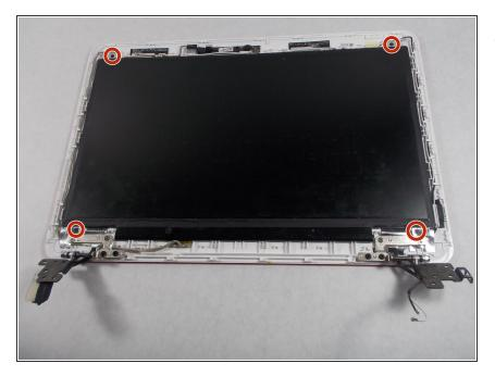
Remove the four 2mm Phillips #0 screws from the four corners of the screen.
