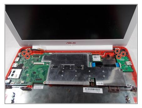
• Unscrew the 6 screws (5 millimeter) on the top right and left.
