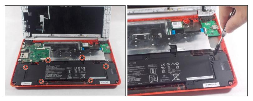
Remove the six 5.6mm Phillips #0 screws around the battery.
