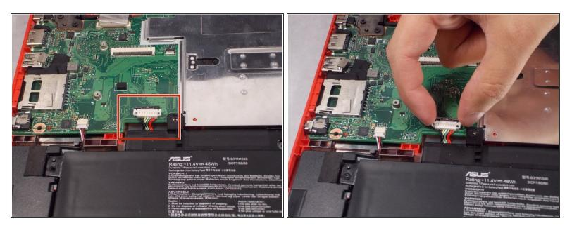
Using your thumb and index finger, pinch the multi-color cable and disconnect it from the motherboard.
