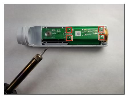
Apply a soldering iron to the mountconnectors and copper-wire connectors until the motherboard can be removed.
