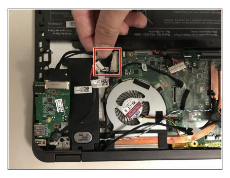
disconnect the cable shown from the motherboard
