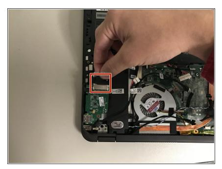
disconnect the cable attached to the top of the USB/SD card/headphone jack interface
