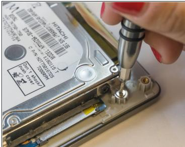
Using the Phillips#00, remove the four 4.5mm screws securing the hard drive.
