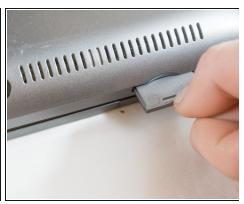
• Using your fingers, pinch the edge of the SD card and pull to remove it.
