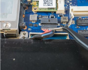
• Using tweezers or your fingertips, carefully pull on the battery connector to disconnect it from the motherboard.
