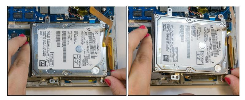
Using your fingers, grasp the edges of the hard drive and lift to remove it.
