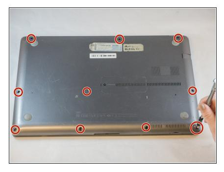
Remove the ten 6.6mm Philips#00 screws securing the lower case to the upper case.
