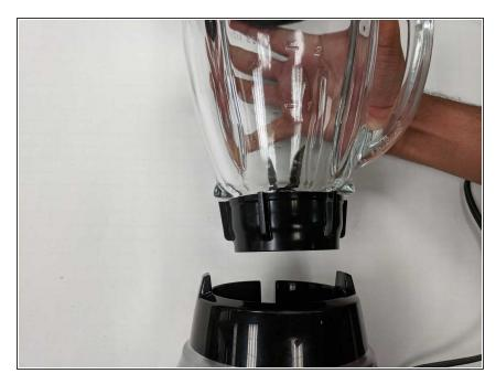
First, remove the blender container from the blender base by grabbing the container and lifting it up.
