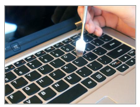
Using a spudger to gently pry up on the selected key until it pops out of its socket.
