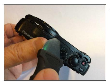
The metal camera front can now simply be pulled off. Ease it on all 4 sides with a spudger
