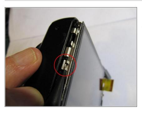
Release a clip on the left hand side of the LCD and hence lift the LCD out.
