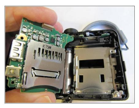
The main logic board can now be removed. It is retained by a clip near the bottom of the left hand side, two plastic pins along the top, and by the connectors which protrude through the right hand side of the camera.
