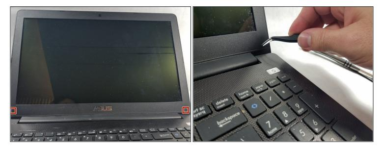
• Using the <u>tweezers</u>, remove the 2 black plastic adhesive covers from the bottom corners of the screen frame.
