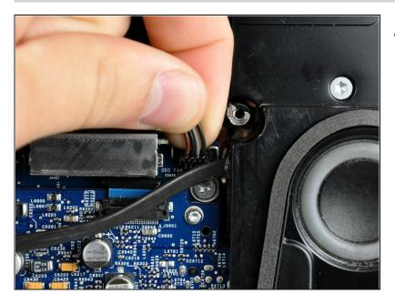
Disconnect the optical drive fan cable connector by pulling it straight up off its socket on the logic board.
