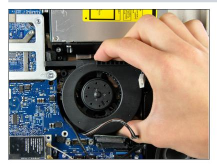
Lift the optical drive fan out of the rear case, being careful not to break the optical drive cable connector.
