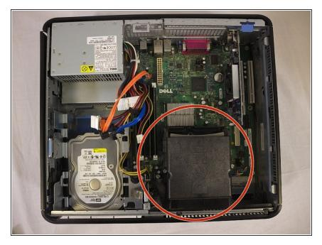
The processor is located inside the heat sink (indicated by the marker).
