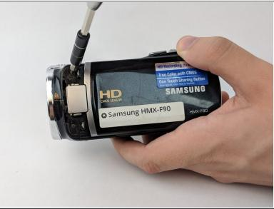
• Locate and remove the two 3.5mm Phillips #00 screws from the side of the camcorder.
