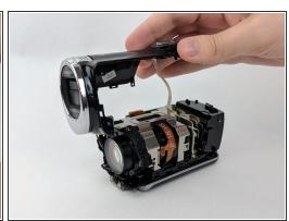
Gradually pry off the outer casing using a prying tool.
