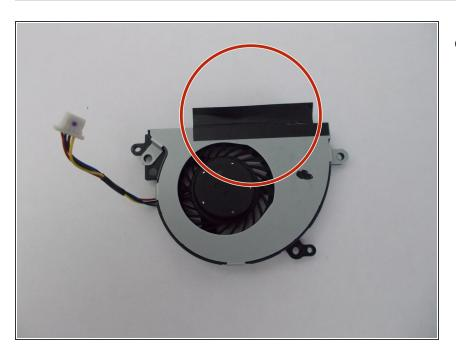
Remove the fan completely . attach electrical tape on the new fan for replacement.
