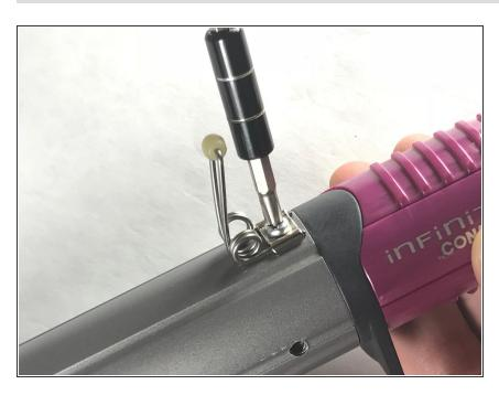
Loosen the spring's Philips #2 13 mm screw.
