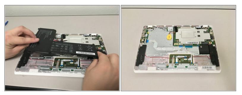
• Lift the battery up and out of the device.
