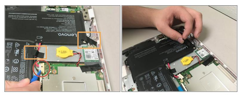
Remove the battery connector from its socket by pulling the cable away from the hinge using your fingers or a plastic opening tool.
