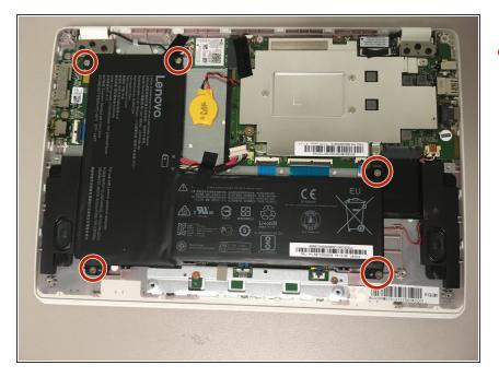
Remove the five 4 mm Phillips screws securing the battery.
