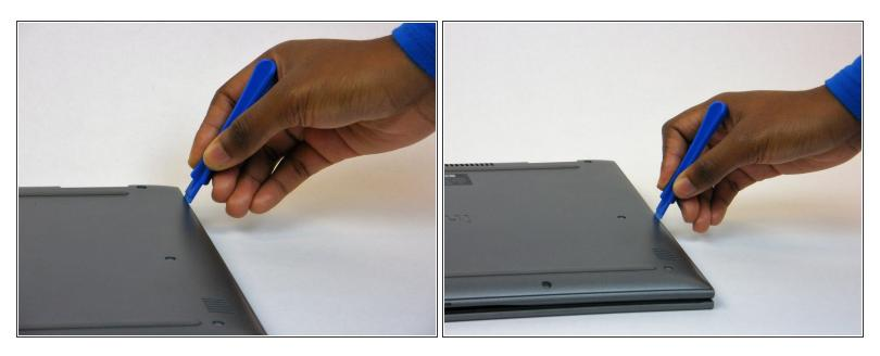
• Use a spudger to pry up and remove the back cover.
