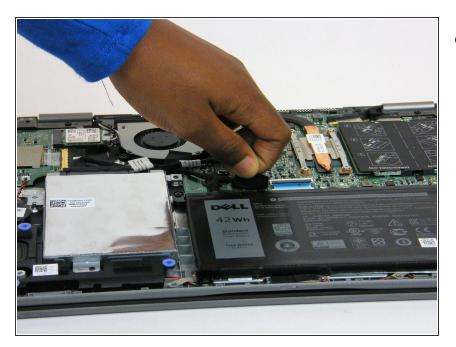
• Pull the battery cable's black tab towards the battery to disconnect it from the motherboard.
