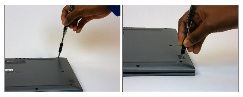
• Remove the nine 6mm Phillips #0 screws that secure the back cover of the laptop.
