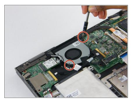
• Remove the 2mm X 3mm screws that are securing the fan.
