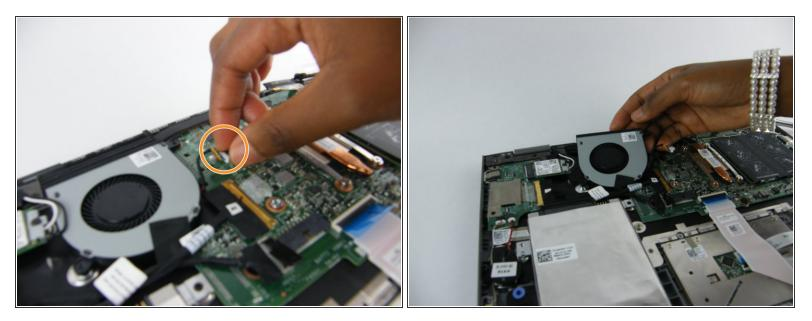
• Unplug the fan from the motherboard, then remove the fan.
