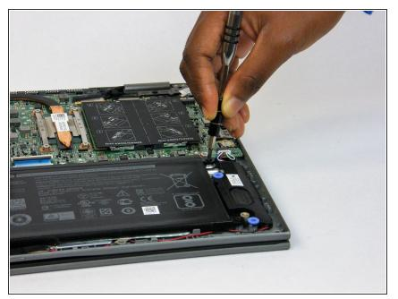
• Remove the four 3mm Phillips #0 screws at the corners of the battery that secure it to the laptop.
