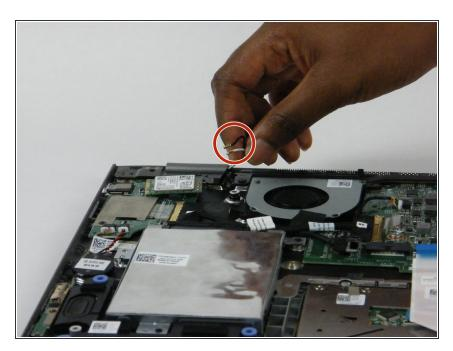
Detach the black and white antenna cables from the WLAN card.
