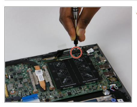
Unscrew the screws that are securing the laptop's hinges.
