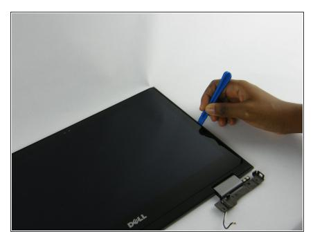
Use your plastic opening tool to pry the LCD back cover from the display panel.
