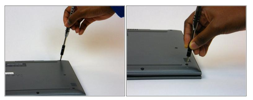
Remove the nine 6mm Phillips #0 screws that secure the back cover of the laptop.
