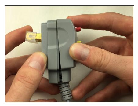
Slide slightly up to remove the back cover of the power plug.
