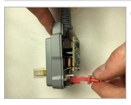
Remove the red reset button by pulling it to the right.
