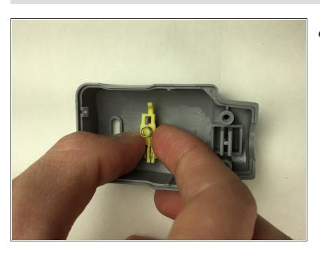
Pull slightly left then up to remove the yellow test button.
