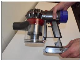
Pull the battery pack down and away from the device.
