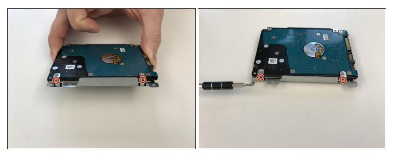
Using a Philip #1 screwdriver remove 2 screws from each side, (removing 4 screws in total) holding the hard drive into the housing.
