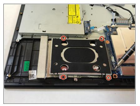
Using a Phillips #1 screwdriver, remove the four (5mm) screws holding the hard drive in place.
