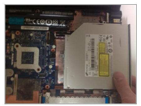
Slide the DVD drive out of the computer to gain access to the cables
