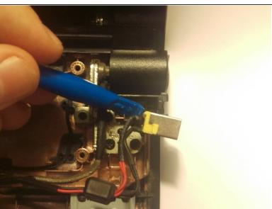
The body of the plug is glued to the computer. Use the spudger tool to wiggle the plug until it comes loose.
