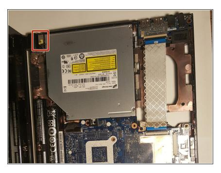
The power connector is easy to spot once you have removed the keyboard.
