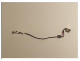
• Use gentle pressure to pull the plug from its socket on the motherboard. Once the plug is loose, you can pull the entire plug assembly from the computer.
