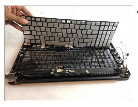
• Lift up the keyboard once it is loosened to remove it.
