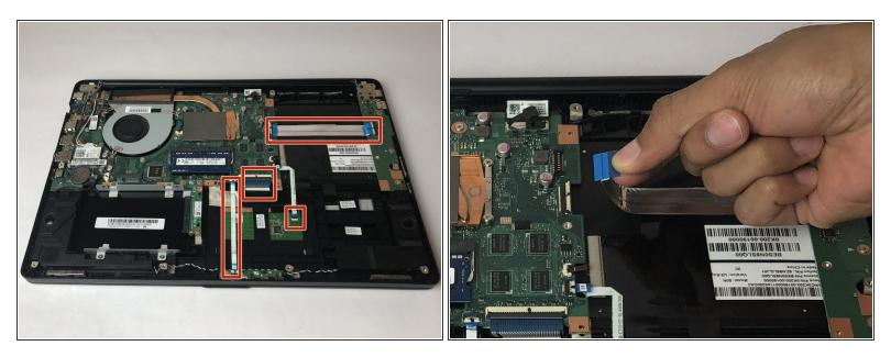
Remove the four ribbons connected to the motherboard.
