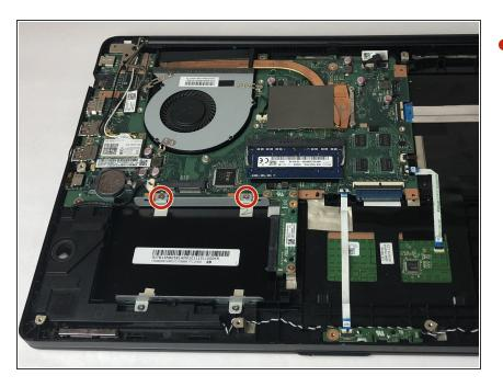
Remove the two 5 mm Phillips #1 screws attaching the stabilizer to the motherboard
