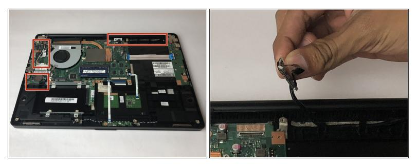
Disconnect the five wires attached to the motherboard by pulling gently. There are three thin wires in the upper left corner.
