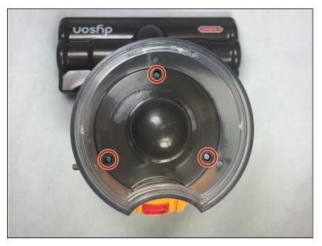
Remove the three 11.5mm (0.45 in) screws at bottom of bead cylinder container using the PH00 screwdriver.
