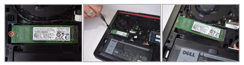
Unscrew the 3mm Philips #1 screw that is holding the SSD in place.
