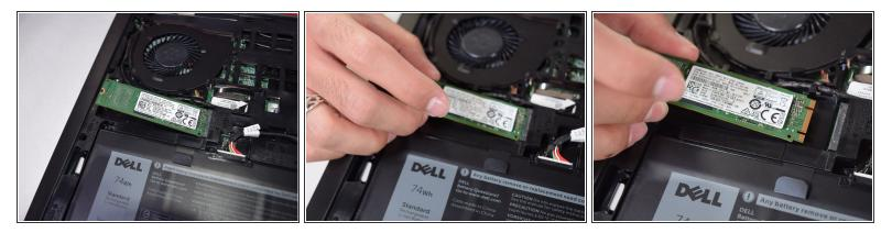
• Gently pull out the SSD, horizontally along the computer to remove it.
