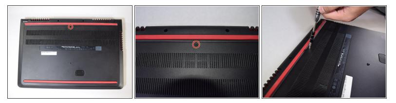
Remove the captive screw located on the top section of the back panel, using a Philips #1 screwdriver.
